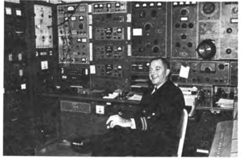
ROBERT J. (Bob) FETZER 2674-V R/O in shack SS CHINA BEAR circa 1966. The China Bear and Philippine Bear were best radio equipped ships, Pgr. or freight ever built by US. Bill Nations of PFEL was responsible for fine gear. Note the large 1KW RCA ET-8063 SSB/CW Xmtr. RTTY is between the TIMES WX FAX Machine and MRT coke box. Antenna patch Jumpers 1st panel at corner left. RTTY TU is next and over to right above 3 Collins Rcvrs is the Times Facsimili converter. Below RTTY TU is Rcr antenna patch board.
